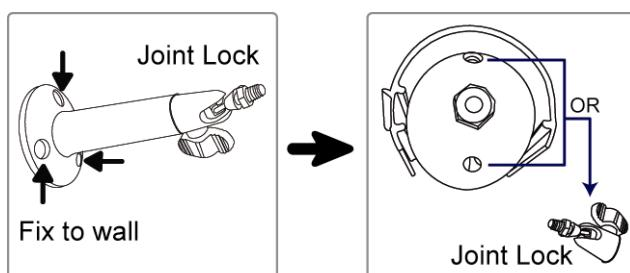
Step3: Fasten the camera with the joint lock to the bracket.
